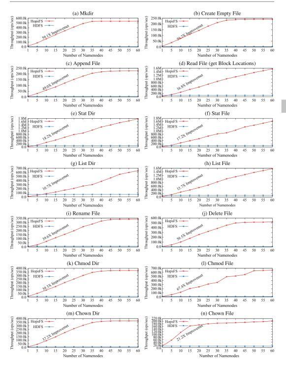
HopsFS: Scaling Hierarchical File System Metadata Using NewSQL Databases, Fig. 6 Throughput of different file system operations in HopsFS and HDFS. As HDFS only supports only one active namenode, the throughput for HDFS file system operations are represented by the
