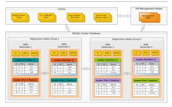
HopsFS: Scaling Hierarchical File System Metadata Using NewSQL Databases, Fig. 3 System architecture diagram of MySQL's Network Database (NDB) cluster.
