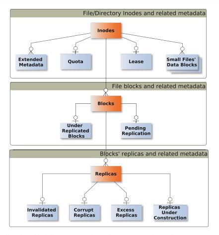
HopsFS: Scaling Hierarchical File System Metadata Using NewSQL Databases, Fig. 5 Entity relational diagram for HopsFS schema
